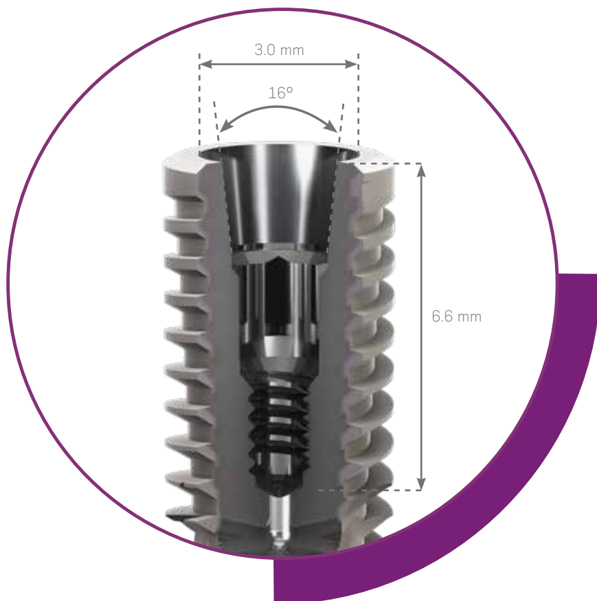
FIGURE 1. The Neodent® Grand Morse® Implant has a deep tapering connection on the inside of the implant, which is designed to increase the contact area between the implant and the abutment. In addition, this connection has a larger diameter, resulting in a simpler, more efficient clinical procedure.
