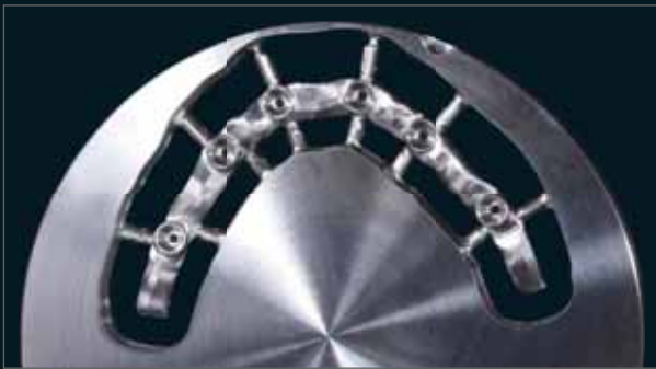
Everything CAD/CAM milled: models, prototype, titanium bar, zirconia structure with threaded screw channels and sealing screws
